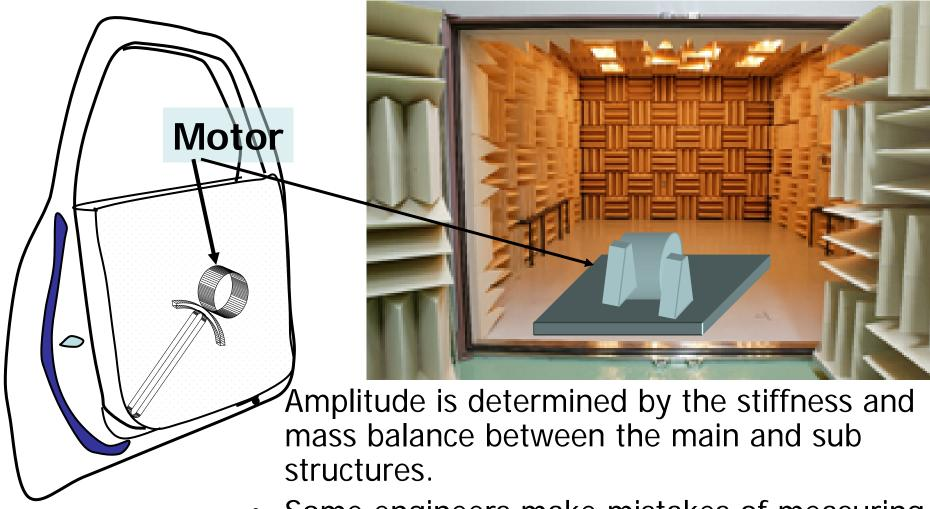
Some engineers make mistakes of measuring noise/vibration in stand alone conditions. Systematic design using coupling parameters as contract conditions
