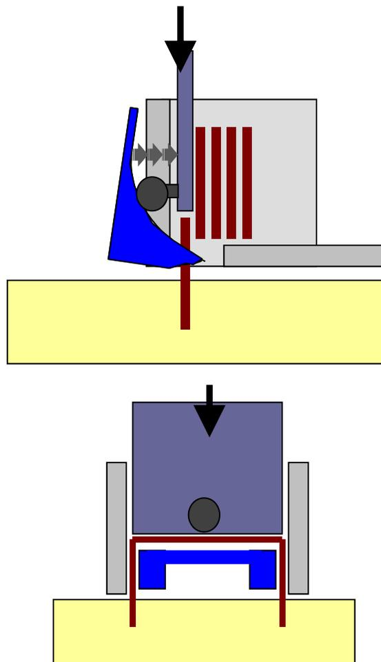
'Little People escape one by one to the front of the stapler' can be realized by 'a triangular supporting part (shown in blue) is pushed forward with the pressing down of the staple.
