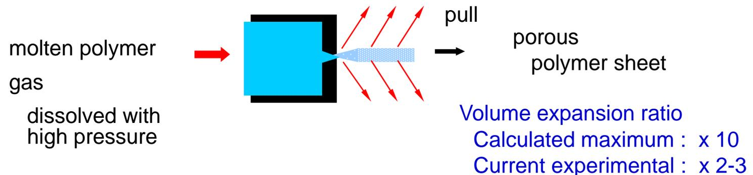
Note: In this slide, technical details (e.g., names of polymer and gas, pressure, mechanism of pushing, etc.) are omitted intently. USIT considers and solve the problem at a conceptual level as shown here.
