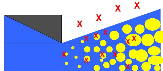
Particles **XXX** are placed outside the polymer surface and inside the polymer, in and around the bubbles.
