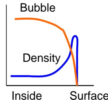
Consideration of the spatial difference in the thickness direction is useful. The polymer is cooled from the surface and gets solid while containing the gas bubbles inside.
