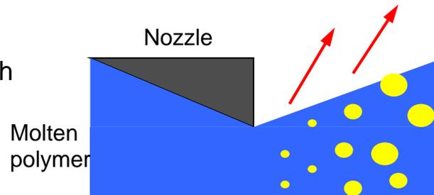
The gas is going out of the polymer surface.
