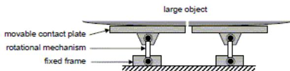
**Fig. 4.** Illustrating orientation of moveable bumper segments to effectively stiffen contact becoming nearly flat.
