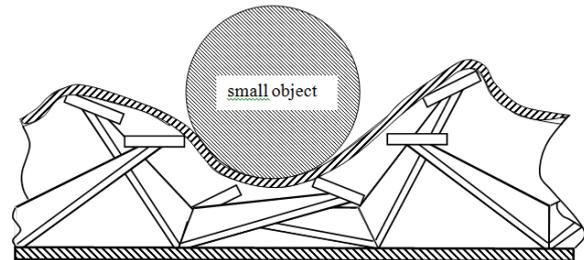
**Fig. 6.** Small object-conformal-shape design. Contact plates now support the conformal material contacting the small object (not to scale).
