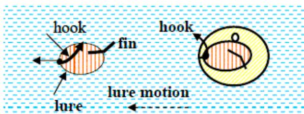
**Fig. 1.** Post solution sketches: Left, moving lure with retracted hook and bent fin. Right, lure enclosed by a fish's mouth, stopping flow, releasing hook, and snaring fish.
