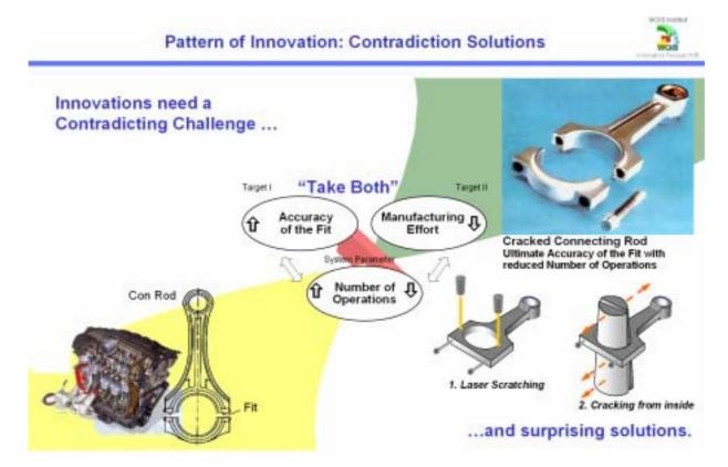
The ever increasing efficiency of engines required the fit of the connecting rod to be machined ever more accurately.
