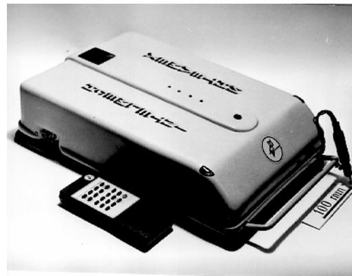
**FIG. 25. Scheme of the climbing robot with middle foot and electromechanical step-by-step drive [6]**
