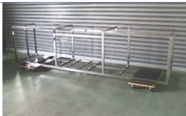
Wildered structure of SUS pipes
