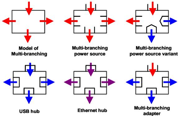
Fig. 9. A connection module with multiple branching: a model and its different examples
