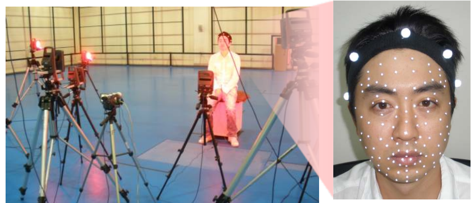
Motion capture device of Vicon co. (Expensive 12 IR cameras are used. About 100 IR markers are attached on face. Several days are needed to clean up the internal noise.)
